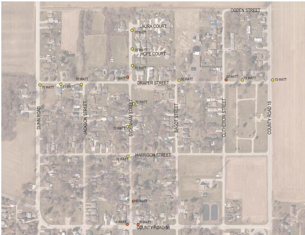
The existing lighting is either 70-73-watt LED (yellow dot) or 50-51-watt LED (orange dot). The streetlights are in a range from 1.5m to 7.0m from the edge of pavement. The streetlights are mounted onto the Hydro One owned wooden poles and have an approximate mounting height of 6.7m (22') above grade, although they do vary.
