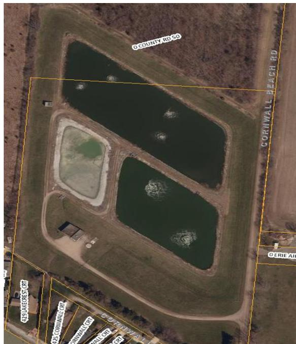
As per ECA number 9096-7SFHHG, the current rated capacity of the Colchester Lagoon is 1,861 m<sup>3</sup>/day. The 2024 average was **953 m<sup>3</sup>/day, or 51% of its rated capacity.**
