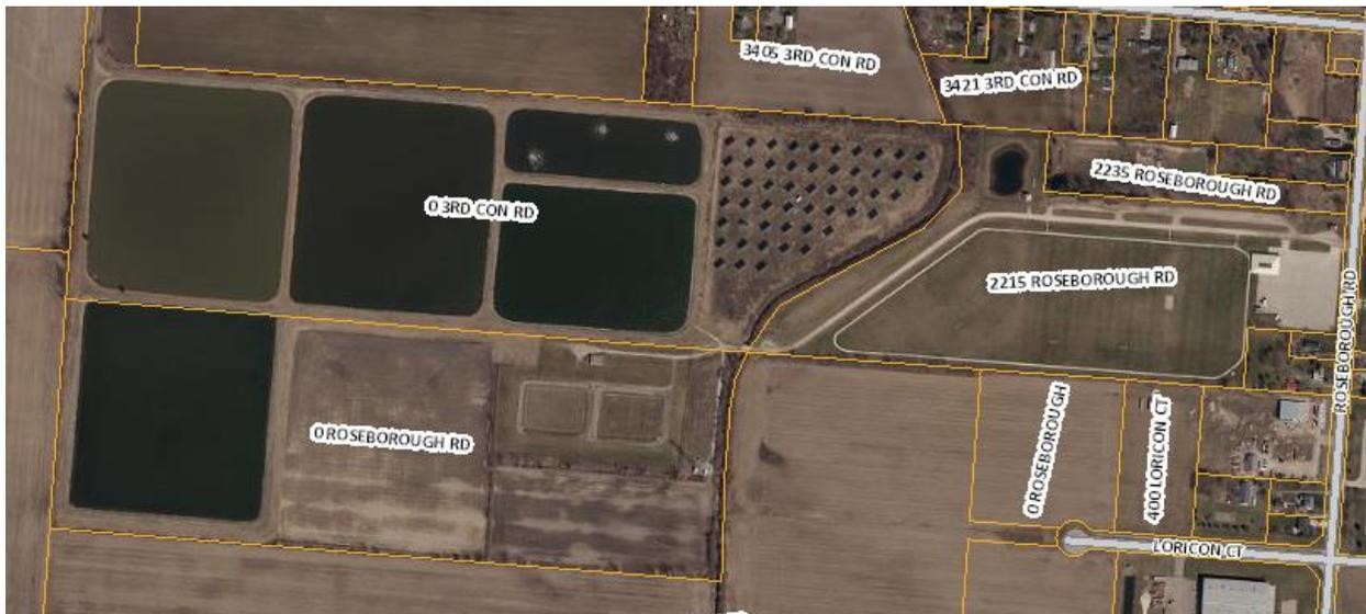
As per ECA number 6365-A4RQ5X, the current rated capacity of the Harrow Lagoon is 2,106 m<sup>3</sup>/day. In 2024, the average daily flow to the facility was **1,034 m<sup>3</sup>/day or 49% of its rated capacity.**
