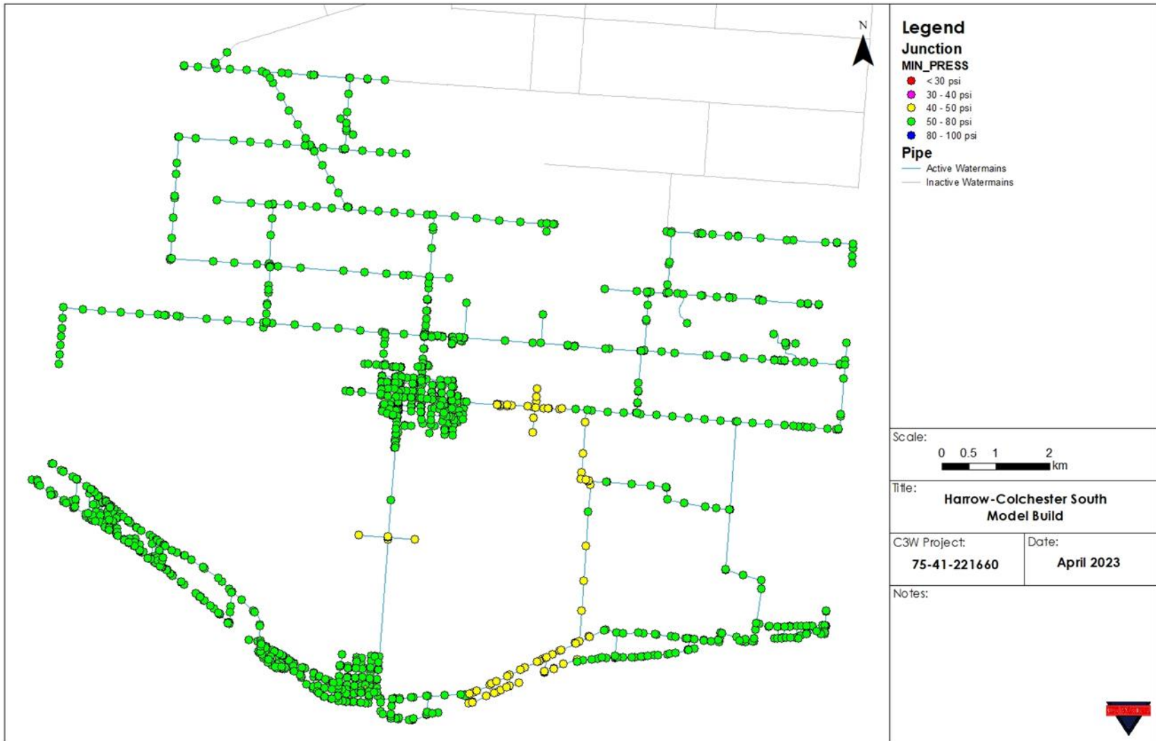
Figure 3-6: HCSWSS Minimum Pressure - MDD 2021
