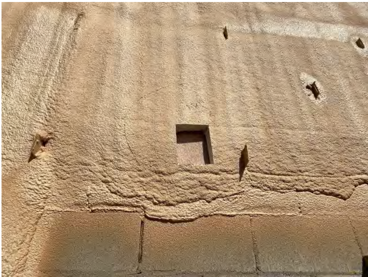
43. Auxiliary Building – Spray Foam Third Party Inspection Hollow Area Marked Out (2022-05-04)
